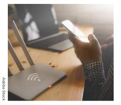
A Wi-Fi router uses radio waves to transmit data to smartphones, tablets, and other wireless devices. Wi-Fi most commonly uses the 2.4 GHz (ultrahigh frequency) and 5 GHz (superhigh frequency) radio bands. A Wi-Fi router using a 2.4 GHz band has a longer transmission range but offers slower data transfer speeds. The 5 GHz band covers a shorter distance but provides faster speeds. A dual-band Wi-Fi router is one that broadcasts radio waves on both bands.
