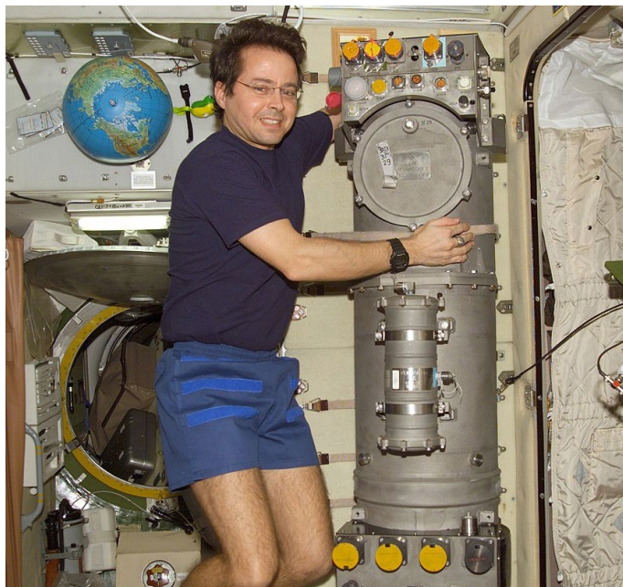
Astronaut Daniel Bursch works on the Elektron Oxygen Generator on the ISS.
