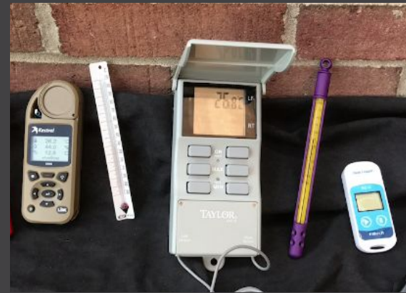
Example thermometers. Credit: GLOBE NOTE: A weather app does not count as “other” - you should have a separate physical thermometer.
