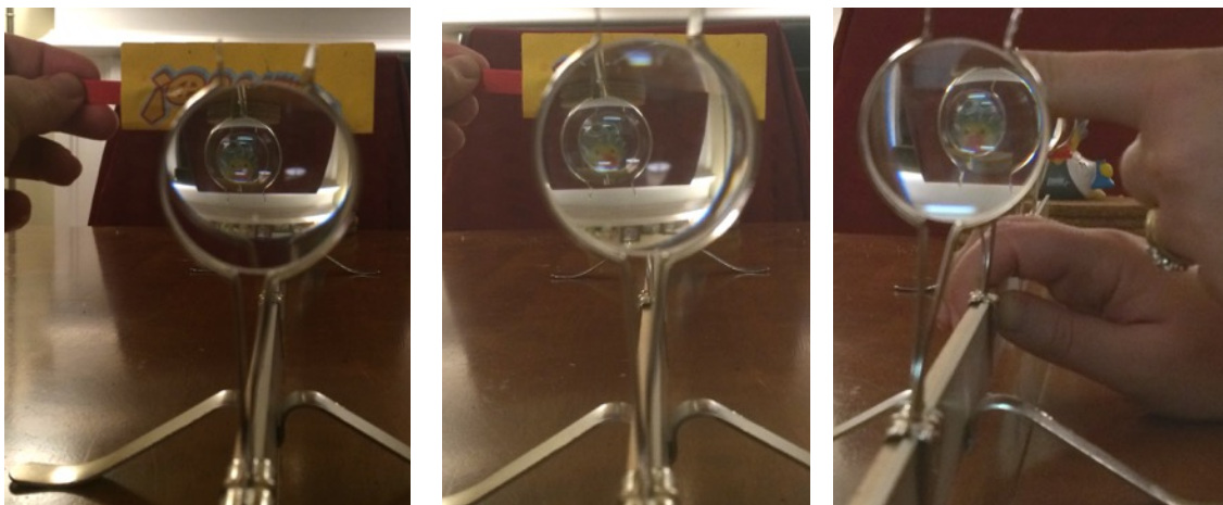
Figure 7. Photos showing the ability of a “Rochester Cloak” to cloak objects
