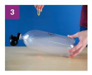
Close the valve and squeeze the bulb 50 times to increase the pressure inside the bottle. Watch the thermometer on the side of the bottle. Does the temperature change as you pump?
