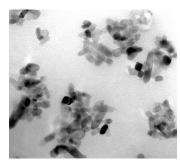
Titanium dioxide nanoparticles Less than 100 nm long
