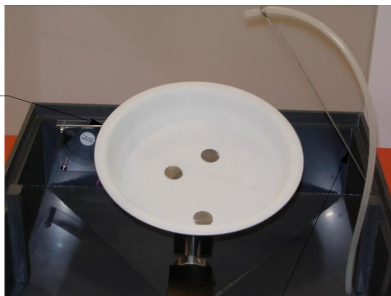
Tube support made from 1/16" Stainless wire. Secured to side of Drain Pan with #6-32 SS screw.
