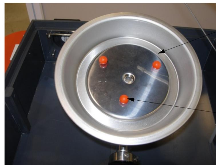
5" 430 SS Wall cover. (McMaster-Carr #2043K23) Secured to pan with Self-Lock Mushroom-Head Fastener (McMaster-Carr #96055K21)
