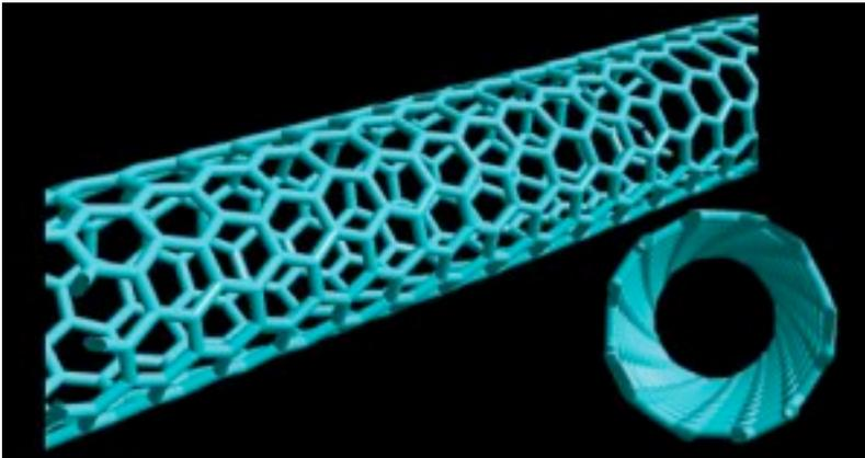
[A carbon nanotube is a hollow tube consisting of repeating hexagonal arrangements of carbon atoms.]
