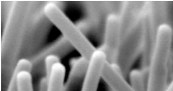
[A scanning electron microscope image of nanowires. Each rod in the image is about 50 nanometers wide.]
