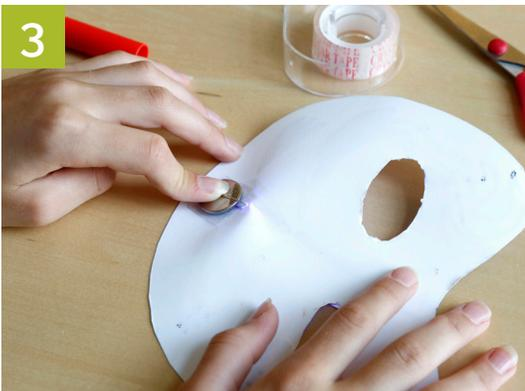
Place the battery onto the tape loop, negative side down. Bend the long leg of the LED onto the top of the battery. The bulb should light up. Tape the top leg and battery down.
